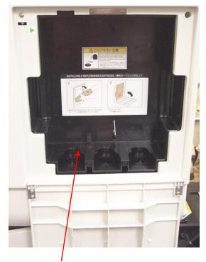
Pour 500 mL of water into this position when making replenisher after completely draining replenisher tanks.
