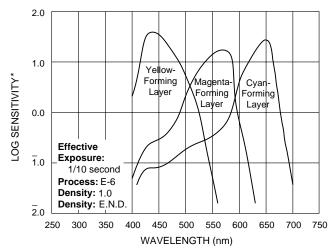
\*Sensitivity = reciprocal of exposure (erg/cm²) required to produce specified density
