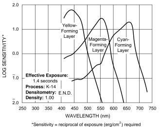
ensitivity = reciprocal of exposure (erg/cm<sup>-</sup>) required to produce specified density F002\_0495AC
