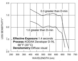
\*Sensitivity = reciprocal of exposure (ergs/cm2) required to produce specified density F002\_0547AC
